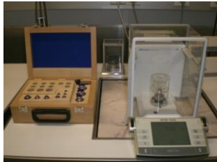
Mass comparator with a maximum range of 20 g and mass standards E2
