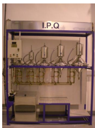
Volumetric standards from 1 L to 20 L
