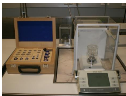
Mass comparator with a maximum range of 20 g and mass standards
