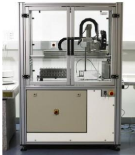
Robotic mass comparator. Resolution: 0.1 µg. Working range: 1 mg to 5 g
