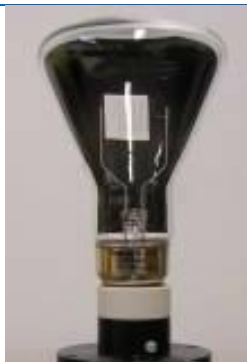
Laboratory standard lamp
